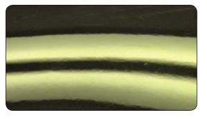
> When the fog is identical everywhere, the dent is repaired.
