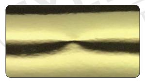
> An outward dent will appear once the lines of the star have been pushed out. Use the knock down on the outward dent, moving the board farther away until the panel returns to its original shape.
