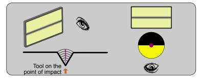
> Position the tool precisely under the point of impact and begin pushing around lightly and playing with the elasticity, relieving the pressure when an outward dent is about to form (up to the elastic limit).
