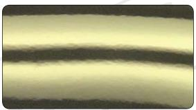
> Once the high spot is tapped down, the panel should be in its original shape. The black line and fog are now identical to an unaffected area of the panel. The dent is repaired.
