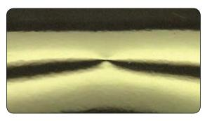
> The dent must be pushed up to create a high spot in order to eliminate the point of impact.
