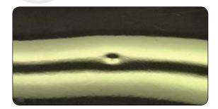
> Small and deep sharp dent. To fix this, we'll use a pointed stainless steel tip.
