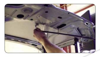
> Leverage must be found for the tool in order to apply steady and continuous pressure on the panel. To apply this pressure, a leverage point is needed, preferably at the midpoint of the tool.
