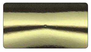
> The dent is deep and very sharp, with reduced elasticity.
