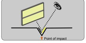
> Proper Board position. Board close in order to see the bottom of the dent.
