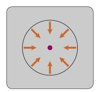
> Do the 1st push, and then proceed in a circle around this point. Continue the spiral pattern in a counterclockwise direction for 3/4 of the dent.
