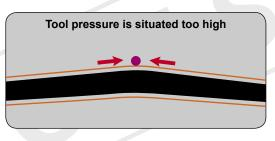
> The indentation doesn't appear yet; the line is bowed too high. The tool is too high (the fog remains the same).
