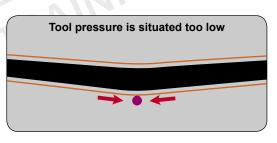
> The indentation doesn't appear yet; the line is bowed too low. The tool is too low (the fog remains the same).
