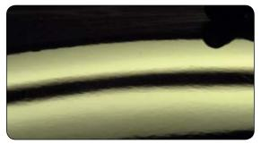
> When the crease is repaired, the black line and the fog must be identical whether in the area of deformation or not.
