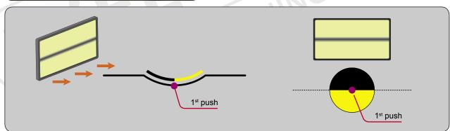
> Position the Board so that you obtain a half yellow/half black line. This will indicate the centre of the dent in a vertical direction; you will then have to centre it yourself in the horizontal direction. Begin to push lightly to see how your dent reacts. You are in the centre of the dent when all the edges of the dent pull towards the centre.
