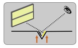
> Poor board position. Board is too far away, bottom of dent not visible, light lines overlap. This will cause you to push off-centre of the bottom and narrow the dent further.
