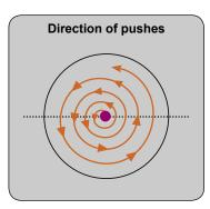
> The same pressure must be applied for each push. The pushes must be connected together so that the orange peel isn't affected. The last quarter of the dent will pop out automatically.
