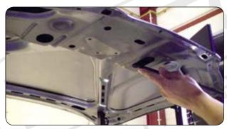
> Direct access through a hole in the brace. Be careful not to deform the inner panels.
