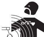
The electric current flowing through any conductor causes electrical and magnetic fields (EMF). The demagnetising current produces an electromagnetic field around the cables and the part to be demagnetised.
