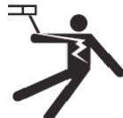
The machine must be connected to an earthed electrical supply. Use the recommended fuse size.
