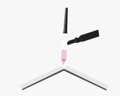
+ 30% more gas consumption In open or flat corner position, the gas escapes on all sides and is therefore less localized in the area to be welded. It is therefore necessary to increase the flow rate.
