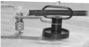
① Weld the earth thanks to contact shrinking tool (p8)
