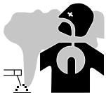
The fumes, gases and dust produced during cutting are hazardous. It is mandatory to ensure adequate ventilation and/or extraction to keep fumes and gases away from the work area. An air fed helmet is recommended in cases of insufficient air supply in the workplace.
