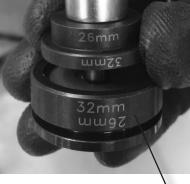
1 upper cutting disc with two diameters: 26 mm at the bottom and 32 mm at the top
