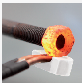
Releasing of rusted bolts
