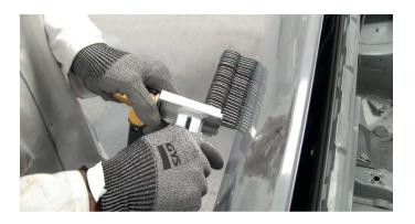
The RINGMATIC can be used with all dent pulling machines with automatic detection in the market using a simple "click" connection.
